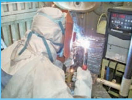
MIG・MAG welding
